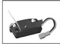
ISH-030-033 2in1 ESC/Receiver unit
