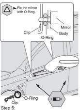
Insert the LED connecting wire and fix the wing mirror with O-Ring on the holes which we drilled in Step 4.
