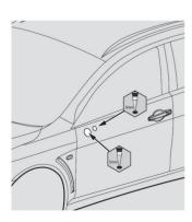
Step 4: We recommend using our body reamer to drill mounting holes.
