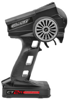
2.4GHz 2-Channel Digital Remote Control System
