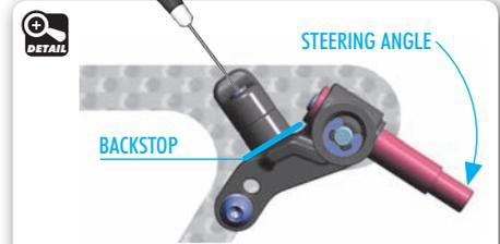
The adjustable backstops are used to limit the steering angle. Adjust the backstop with the set-screw to achieve the maximum steering angle needed. Adjust the steering angle on both L & R sides to the same amount.
