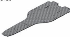
The 2.5mm chassis made from harder graphite material was developed for very-high traction conditions, or when using tires that offer a lot of steering which makes the car more difficult to drive. This chassis makes the car more stable and easier to drive, and eliminates oversteering.
