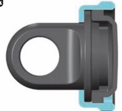
After you insert the membrane, ensure that it is fully seated inside the alu cap.
