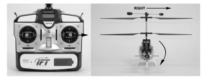
The aileron trim lever (located immediately below the right-hand stick) can be used to help keep the helicopter from drifting left or right when hovering and with no right-hand stick/aileron control input. For example, if the helicopter drifts to the right when hovering slide the aileron trim lever to the left until the helicopter hovers as level as possible without drifting to the right.
