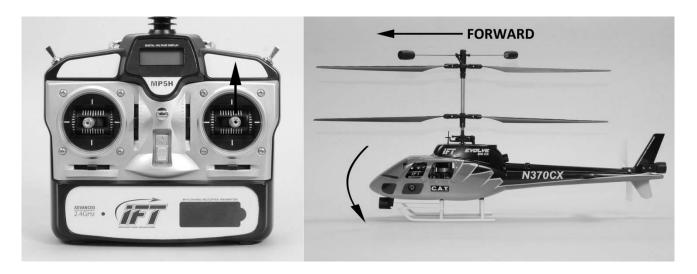
Pulling the right-hand stick downward/backward will pitch the tail of the helicopter downward, allowing it to be flown backward. This is accomplished by having the elevator (left-hand) servo pull the swashplate downward.
