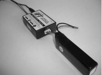
□ When the battery is connected to the charger securely and with the proper polarity both the red color and green color LED indicators will glow solid. The battery will be charging anytime the green LED indicator is glowing solid.
