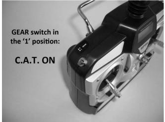
When using your transmitter/receiver of choice with the RFR version you can turn the technology on and off using the suitable 2-position switch (recommended), 'slider' switch or rotating knob for the channel you connected the 'Gear' lead to when installing the receiver. Please see the 'Installing the Receiver' section of this manual for more information if needed.
