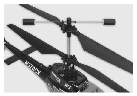
To install the factory-assembled short length stabilizer flybar set/assembly start by first removing the two small screws that hold the cap/cover to the top of the upper rotor head/hub. Slide the cap/cover out of the head/hub and set it to the side. Now you can remove the standard length stabilizer flybar and disconnect the ball link/linkage from the main rotor blade grip.
