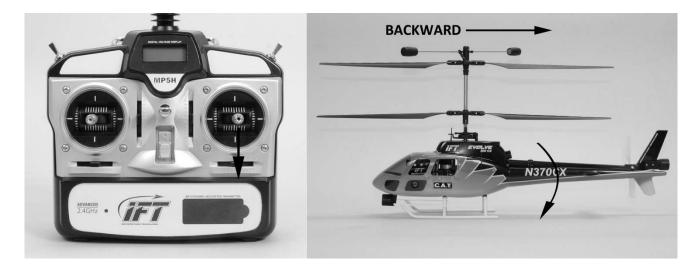
The elevator trim lever (located immediately to the left of the right-hand stick) can be used to help keep the helicopter from drifting forward or backward when hovering and with no right-hand stick/elevator control input. For example, if the helicopter drifts forward when hovering slide the elevator trim lever downward until the helicopter hovers as level as possible without drifting forward.
