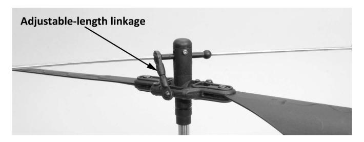
You can check the upper main rotor blade tracking with the helicopter on the ground or in the air while flying. Also, we recommend having an assistant on hand to help 'sight' the blades (especially if you'll be checking the blade tracking while flying).
