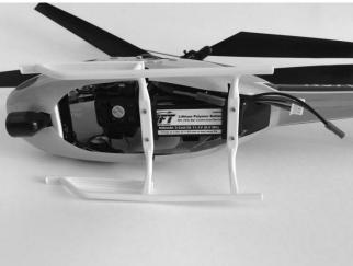
QUICK TIP: If you find it difficult to install and remove the battery you can use scissors (we recommend 'lexan' type scissors available from most hobby shops) and/or a sharp knife (and extreme care to prevent personal injury!) to remove material and make the opening in the body wider and longer.
