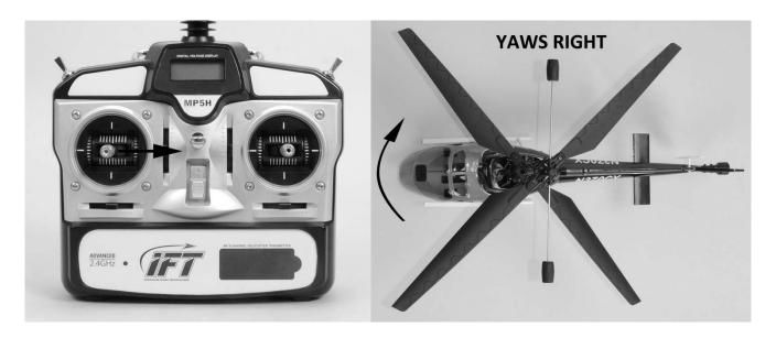
The rudder trim lever (located immediately below the left-hand stick) can be used to help keep the nose of the helicopter from turning (yawing) to the left or right when 'hovering' and without any left-hand stick/rudder control input. For example, if the nose of the helicopter turns to the right when hovering slide the rudder trim lever to the left until the nose of the helicopter stays as close to 'straight' as possible with no further rudder control/trim input.
