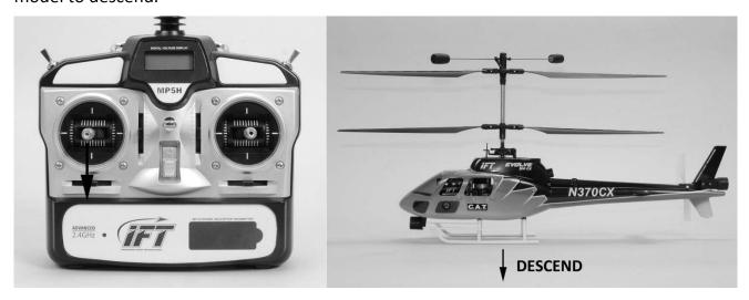
After lifting the helicopter off the ground you can maintain altitude in 'hover' by carefully moving the left-hand stick up and down slightly as needed so the helicopter will not climb or descend.
