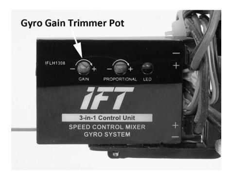
• The gain value is set too high if the nose/tail of the helicopter twitches quickly from side to side when in hover and/or fast forward/backward/sideways flight. If you find this to be the case for your helicopter, decrease the gyro gain value in small increments until the nose/tail of the helicopter no longer twitches quickly from side to side.
