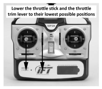
Moving the left-hand stick to the left will turn (yaw) the nose of the helicopter to the left about the axis of the main shaft. This is accomplished by increasing the speed/RPMs of the lower set of main rotor blades while decreasing the speed/RPMs of the upper set of main rotor blades.
