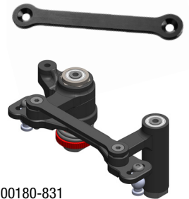
C-00180-831 Steering Rack - Dual Stiffener - Alumin- ium - 1 Pc
