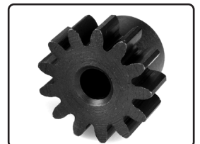
C-72815 M1.0 Pinion - 15T - Hardened Steel - Shaft Diameter 5mm
