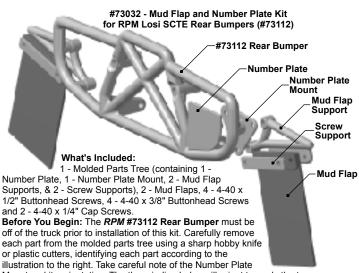
Mount and its orientation. The three in-line holes will orient towards the top. Take note of the "NP" label. The two mounting screws for the number plate will enter from these two holes.
