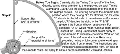
**Step #1:** Slip the *RPM* Prop Guard over the top of the gearbox and orient it so the support bars of the Guard point straight out of the front (or rear) of the airframe and 90° to the side.
