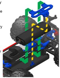
connect the battery pack to the ESC at this time.
