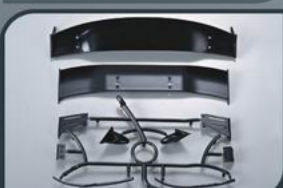
48128 Rear Wing (injection molded) Used with 1/10 RC car
