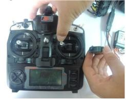
Double adjust the servo to ensure horizontal position for smooth operation. Please operate this way during future use, as required.
