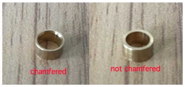
Get it through 1 (Bushings have a chamfering on one end. The chamfering end must be installed towards the nozzle direction to avoid tube from bursting. Follow the same method for next following assemblies).
