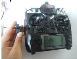
Try to keep the servo arm in the horizontal position as shown
