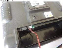
Connect power cables (Note: The cable of positive pole (Red line) must be in the middle position)
