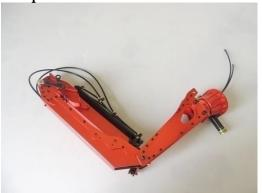
Pull out two tubes (Note: These two tubes are used for hook, please make a mark for future assembly)
