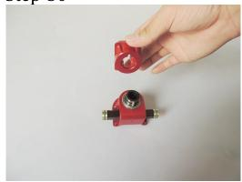
Align the position between key way and key
