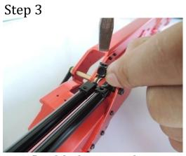
Use flat-blade screwdriver to install 2 onto cylinder
