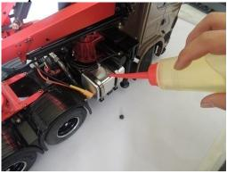
Add 150ML hydraulic oil then close the cap (Turn on the pump while adding hydraulic oil).
