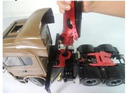
Put oil tube into the hole (Be careful to avoid damaging the oil tube)
