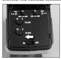
1. Switch radio on. (ALWAYS turn your radio 2. Install the battery into the vehicle and on first!)
