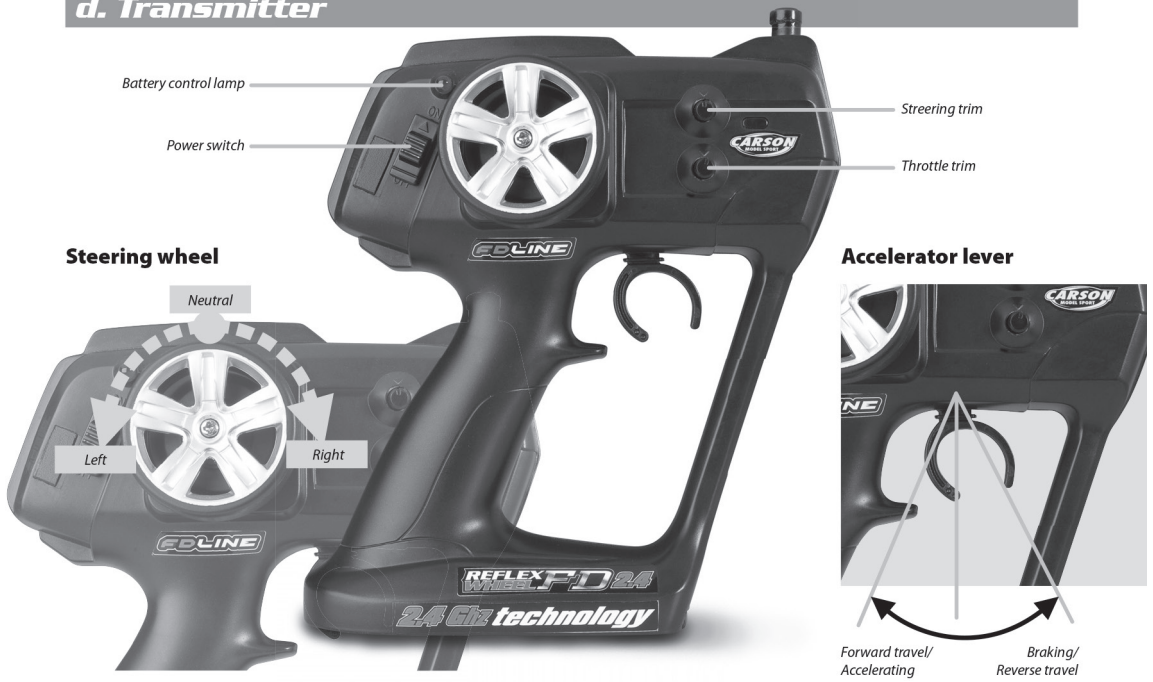
The more you turn the steering wheel, the greater the head angle of the front wheels.
