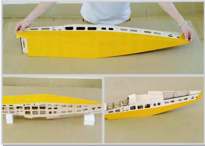
9.5 Iron on covering for the side panels. Always use lower heat to stick on the covering. Use high heat carefully only for shrinking covering around corners.
