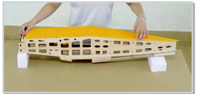
11.3 Place covering on fuselage bottom, completely covering the surface with 5mm overhang at all sides.
