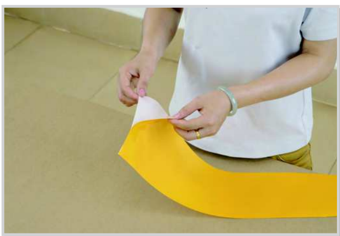
9.2 Take out the covering piece for the bottom of fuselage, and peel off backing sheet.
