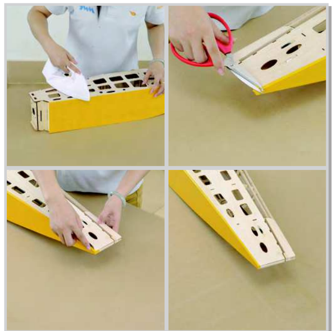
9.4 Iron on the overhangs to cover the edges. If you need to shrink the covering to conform to the shape of edges, you can do so by raising the iron temperature. Just apply heat at the required spot only. Since the shrinking temperature is much higher than the adhesive melting temperature, if you apply high heat at area near the edge or seams of covering, the covering will pull away from the edge or seams. Trim off unwanted material.
