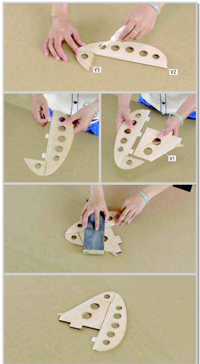
6.1 Place V2 and V3 on flat surface and apply glue to glue them together. Insert CA hinges to the vertical stabilizer hinge grooves, install rudder and check alignment of rudder. Do not apply glue to the CA hinges at this stage. Sand down rough edges if necessary.
