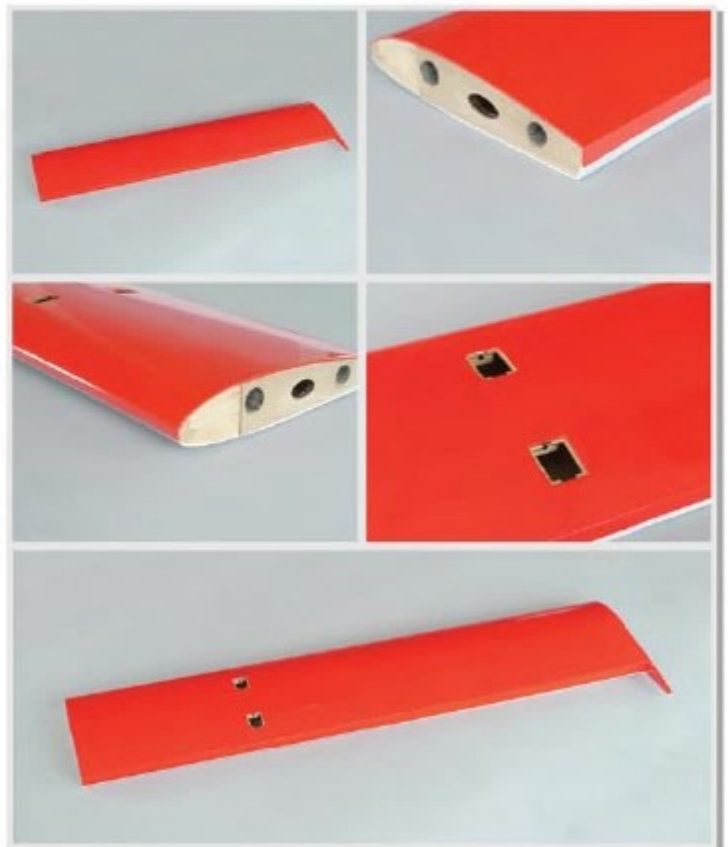
6.22 Cover top of wing. Allow 3 mm overlap at both ends and total 6 mm overlap at leading edge. Cut openings for wing tube latch hatch.
