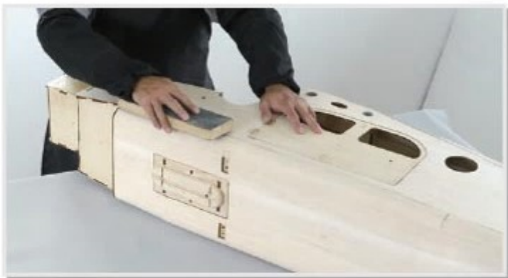
4.31 Remove rough edges with sand paper.
