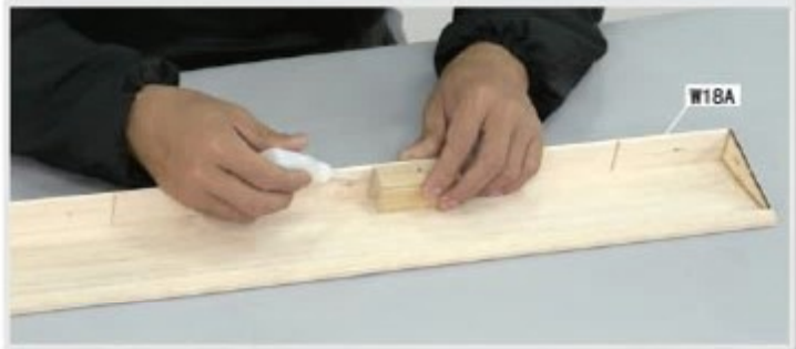
1.29 Glue W25A in place at both ends. Glue W31 to W35A opening, then glue W18A in place. Make sure W31 tapers towards the trailing edge.
