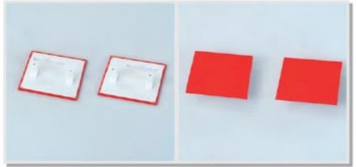
6.11 Cover the aileron servo tray.
