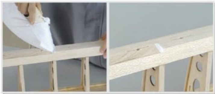
6.19 Cover wing hinge beam.
