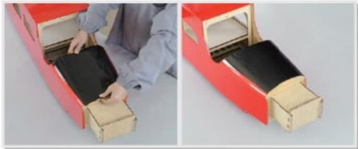
6.9 Cover the battery hatch.
