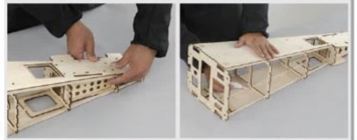
4.4 Glue in F9C, F10, F11 and F12, then glue in the right side panel. Make sure all the latches are fully inserted into corresponding slots.
