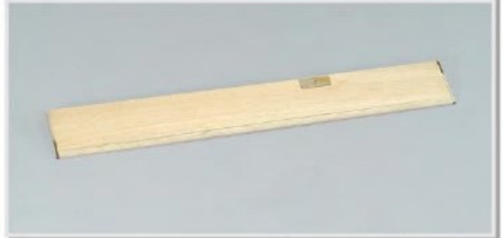
1.33 When cured, remove rough edges with sand paper.
