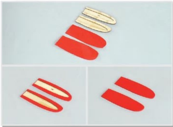
6.17 Cover elevator end plate.
