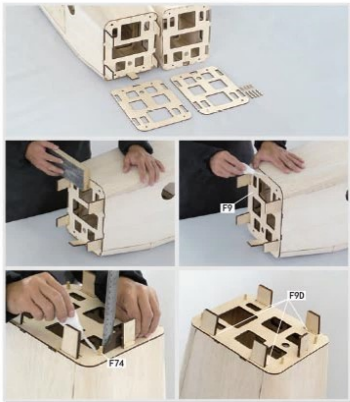
4.33 Glue on F9 to fuselage front section. Glue in F74, use set square to make sure F74 is perpendicular to F9. Glue in F9D.
