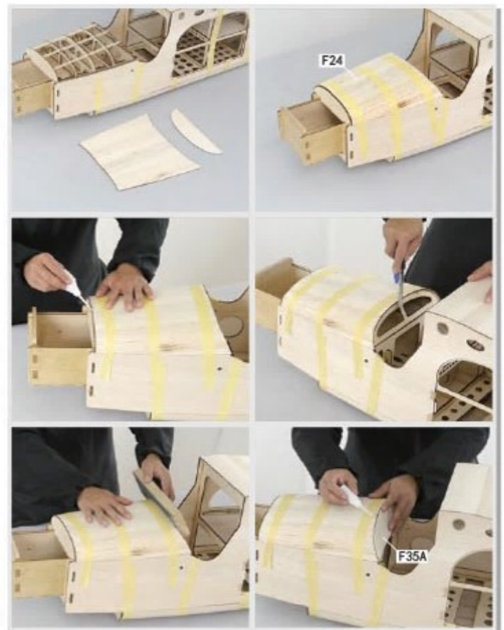
4.29 Apply slow curing glue to surfaces in contact with F24. Apply moisture to outer 6 cm portion of F24 then put on top of frame. Use tape to hold F24 in position. When cured remove rough surface by knife and sand paper. Glue in F35A.
