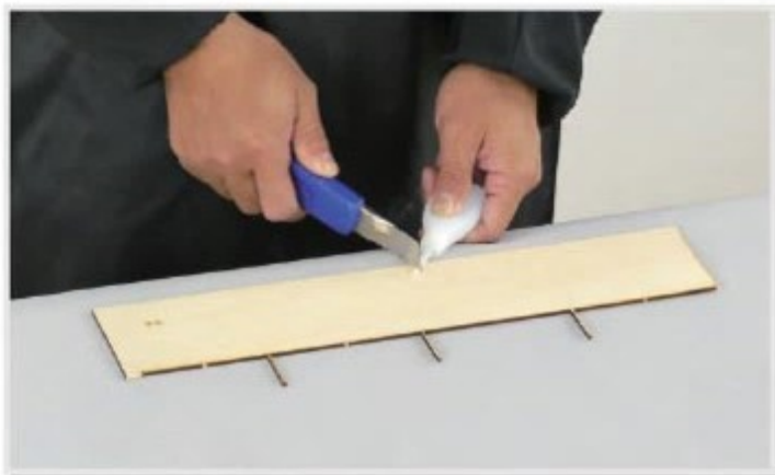
1.2 Cut open CA glue tip for CA application. Make sure opening is not pointing at anyone.
