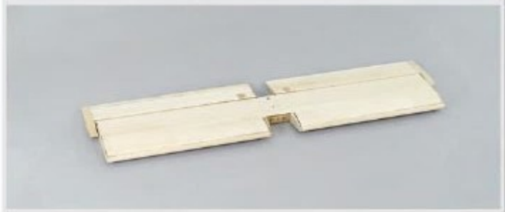
2.14 Connect elevator and horizontal stabilizer with align-pro hinges.
