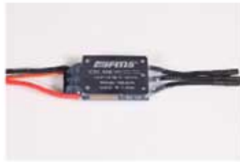
FMS-ESC-70A with 5A SBEC
