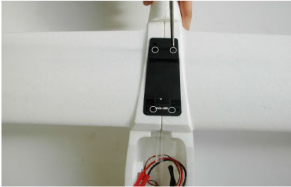
6. Secure the main wing. Screw-PM3.0*45(4PCS)
