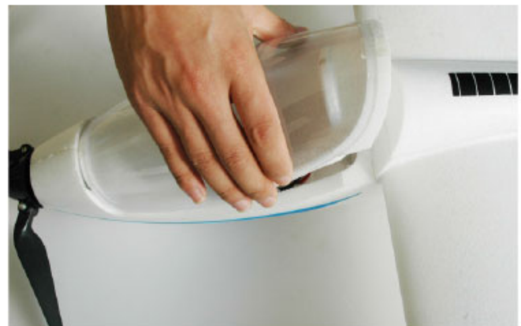
11. Install the canopy.
