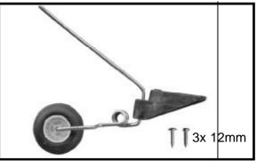
□ 2. Using a pen, mark the locations of the two mounting screws. Remove the tail wheel bracket and drill 1mm pilot holes at the locations marked.
