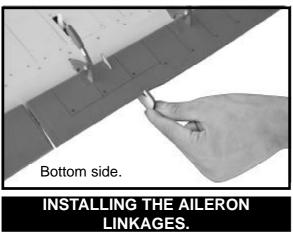
Installing the aileron linkages as pictures below.
