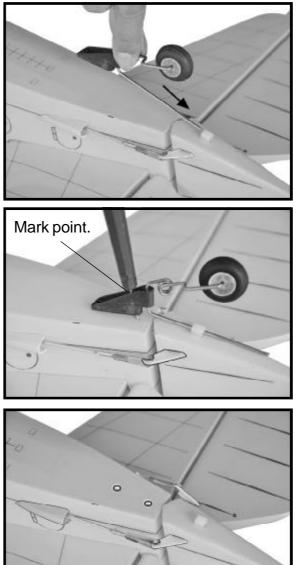
$\Box$  3. Secure the tail wheel bracket in place using three 3mm x 12mm wood screws. Be careful not to overtighten the screws.
