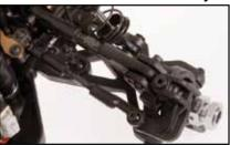
Wheel-axles and driveshaft front
