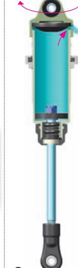
**5** Gently place the shock cap assembly onto the filled shock body. Excess oil will spill from the shock. Screw the shock cap onto the body by only a few turns.
