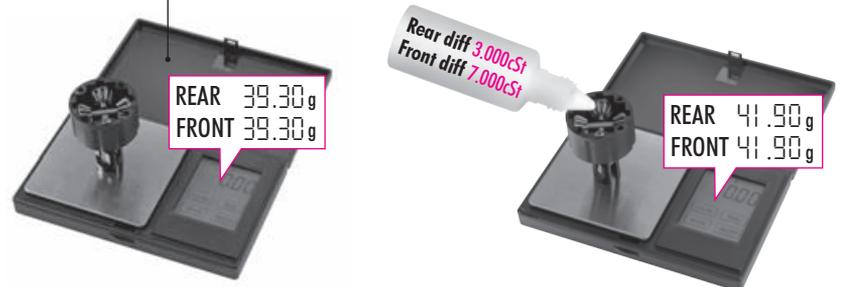
1. Put the diff (without oil) on the scale and check the weight:
