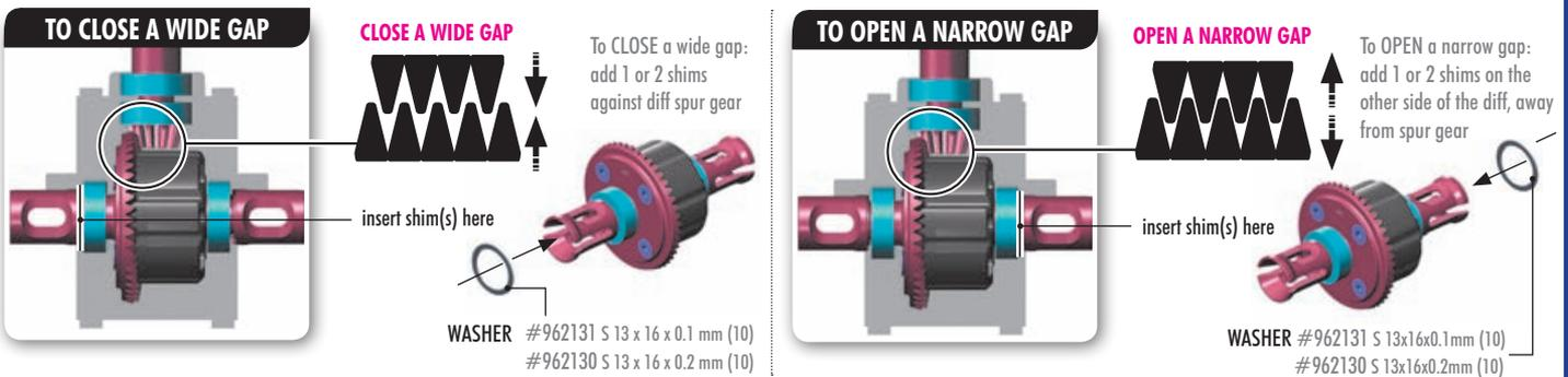
**CHECK GEAR MESH AND DIFF PLAY ONLY AFTER THE ENTIRE GEARBOX IS MOUNTED TOGETHER WITH THE SUSPENSION HOLDERS ON THE CHASSIS. ALL PARTS ARE DESIGNED TO HAVE CERTAIN PLAY AND IT IS ALL DESIGNED BY PURPOSE.**
