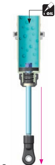
**1** Extend the shock shaft completely. Fill the shock body with the shock oil. For the FRONT shocks (short) use 550cSt oil. For the REAR shocks (long) use 600cSt oil.
