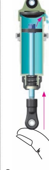
**6** Gently push the shock shaft completely into the shock body. Excess oil will flow through the hole in the shock cap.
