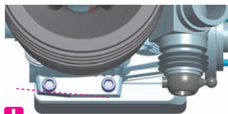
When installing the engine, first check that the drive shaft does not touch the engine. If it does, remove some material from the engine mount as shown to make some room between engine and shaft.
