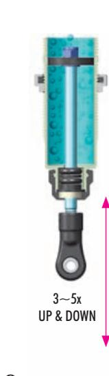
**2** Move the shock shaft up and down a few times to release the air bubbles trapped beneath the piston.
