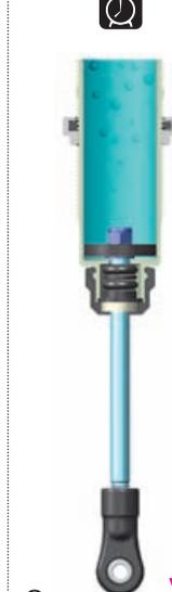
**3** Orient the filled shock vertically for several minutes with the shock shaft fully extended. The remaining air bubbles will release.
