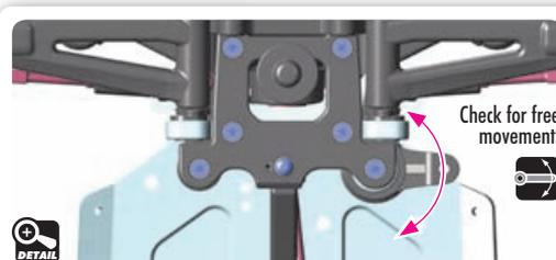
After the top deck assembly check for free movement of steering system.
