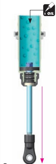
1 Extend the shock shaft completely. Fill the shock body with the shock oil. For the shocks use 800cSt oil.
