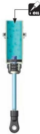
2 Fill the shock body with shock oil up to the top. Make sure to use same viscosity shock oil as is in the shock.
