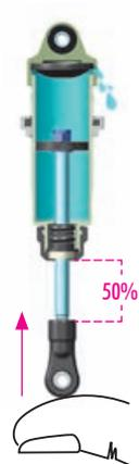
5 Push the shock shaft 50% into the shock body. Excess oil will bleed through the hole in the shock cap.
