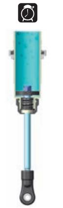
3 Orient the filled shock vertically for several minutes with the shock shaft fully extended. The remaining air bubbles will release.
