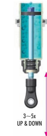
2 Move the shock shaft up and down a few times to release the air bubbles trapped beneath the piston.
