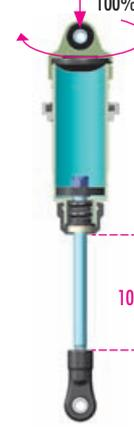
4 Gently place the shock cap assembly onto the filled shock body. Keep the shock shaft extended 100% from the shock body and tighten the shock cap completely. The rebound will be at approximately 100%.
