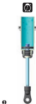
3 Orient the filled shock vertically for several minutes with the shock shaft fully extended. The remaining air bubbles will release.
