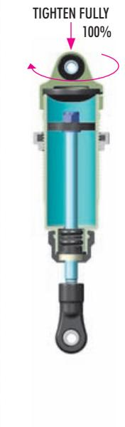
7 Keep the shock shaft pushed in the shock body and tighten the shock cap completely. The rebound will be at approximately 0%.
