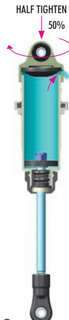
5 Gently place the shock cap assembly onto the filled shock body. Excess oil will spill from the shock. Screw the shock cap onto the body by only a few turns.
