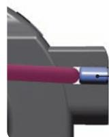
Step 1 Loosen the 3x5 setscrew if the anti-roll bar does not turn freely.
