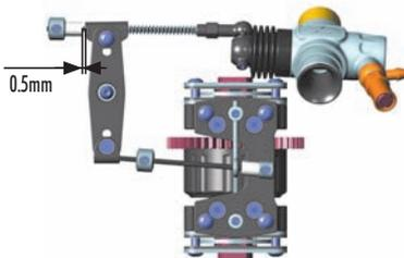
Turn on the transmitter and receiver and set the engine control servo trim to the neutral position. Adjust the idle adjustment screw on the carburetor to open approx. 1mm. Adjust both the throttle linkage and brake linkages accordingly. DO NOT adjust the linkage with the engine running.
