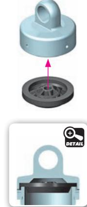
**4** Install the shock membrane into the groove in the upper shock cap.
