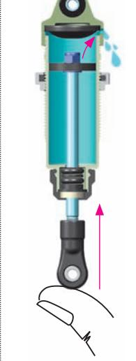
**6** Gently push the shock shaft completely into the shock body. Excess oil will flow through the hole in the shock cap.
