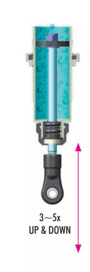
**2** Move the shock shaft up and down a few times to release the air bubbles trapped beneath the piston.
