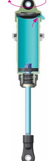
**5** Gently place the shock cap assembly onto the filled shock body. Excess oil will spill from the shock. Screw the shock cap onto the body by only a few turns.
