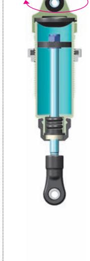
**7** Keep the shock shaft pushed in the shock body and tighten the shock cap completely. The rebound will be at approximately 0%.
