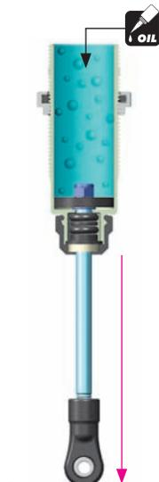
**1** Extend the shock shaft completely. Fill the shock body with the shock oil. For the FRONT shocks (short) use 550cSt oil. For the REAR shocks (long) use 450cSt oil.
