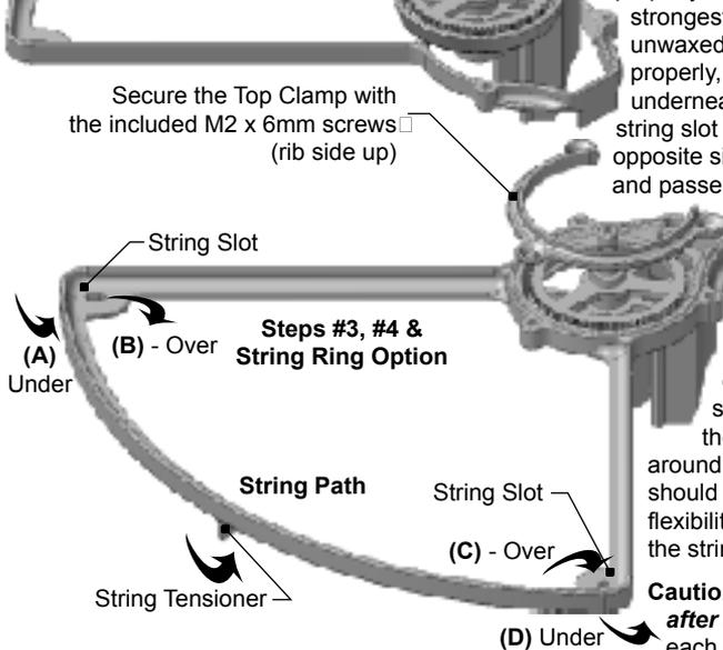
Once the string has been threaded through, pull it around the string tensioner (on the bottom of the Prop Guards) on 2 of the 4 Prop Guards. Tie the string with **at least** a double knot, then tension the string by slipping it around the last 2 tensioners. The string should be tight enough to allow some flexibility of the guards without allowing the string to come loose.
