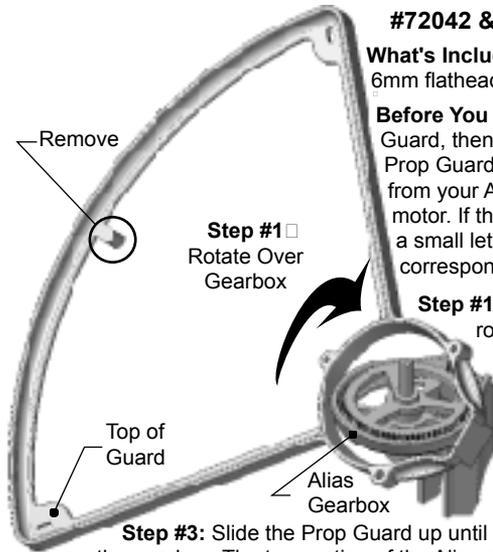
**Step #1:** Slip the **RPM** Prop Guard over the gearbox, rotating it vertically to allow it to "roll" over the top of the gearbox. Caution: The top of the Prop Guard must face outwards (see illustration) for the correct orientation once it's installed.
