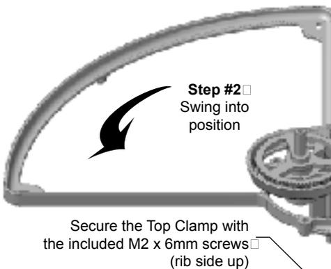
**Step #4:** Using the included screws, attach the Top Clamp to the Prop Guard with the **rib side up**. Caution: Do not overtighten the screws.
