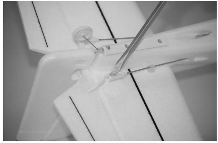
After connecting the clevises to the control horns view the vertical tail and rudder from directly above. The rudder should be 'in line' with the vertical tail when it's properly 'centered'. However, if the rudder is angled off to the right or left you can adjust the length/position of the pushrod/clevis so the surface is centered 'mechanically' while the trim lever on the transmitter is centered.
