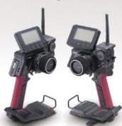
This unit is comprised of the throttle and power. 4 x AA batteries are needed and the battery magazine is inserted into the grip. A left-handed version will also be available.
