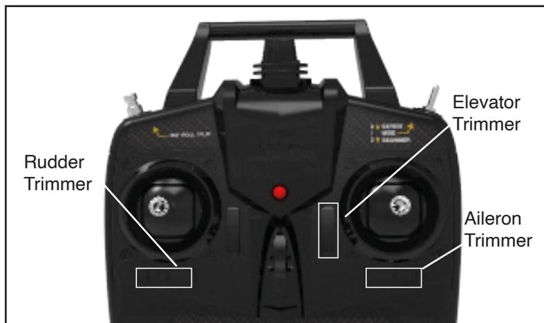
Digital trims allow to adjust the centered position of aileron, rudder or elevator hinge. Each time when a trimmer is moved, the servo output will change one angle. If the trimmer is held, the output will scroll in that direction until the trimmer is released or the output reaches its end. When you hear a short "beep" sound, it means the trimmer is centered.
