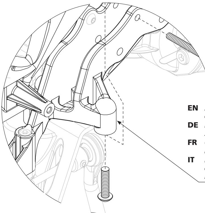
**EN** Spread the lower portion of the cage assembly open to clear the screw boss when assembling.
