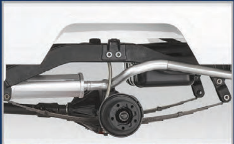
Rear Suspension: Leaf springs w/damper cylinder
