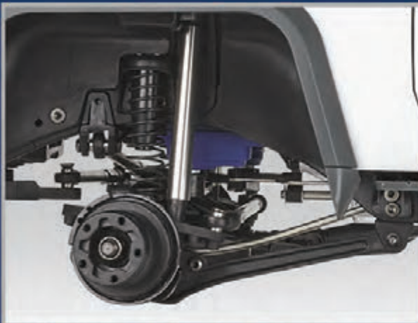
Front Suspension: 3-linkage suspension w/coil springs
