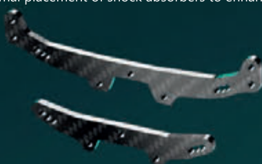
3.0MM ECO-GRAPHITE F/R LCG SHOCK TOWERS
