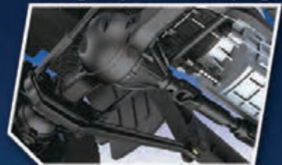
Rear suspension: Leaf spring w/damper cylinder
