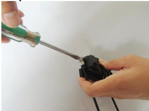
Use flat-blade screwdriver to assemble
