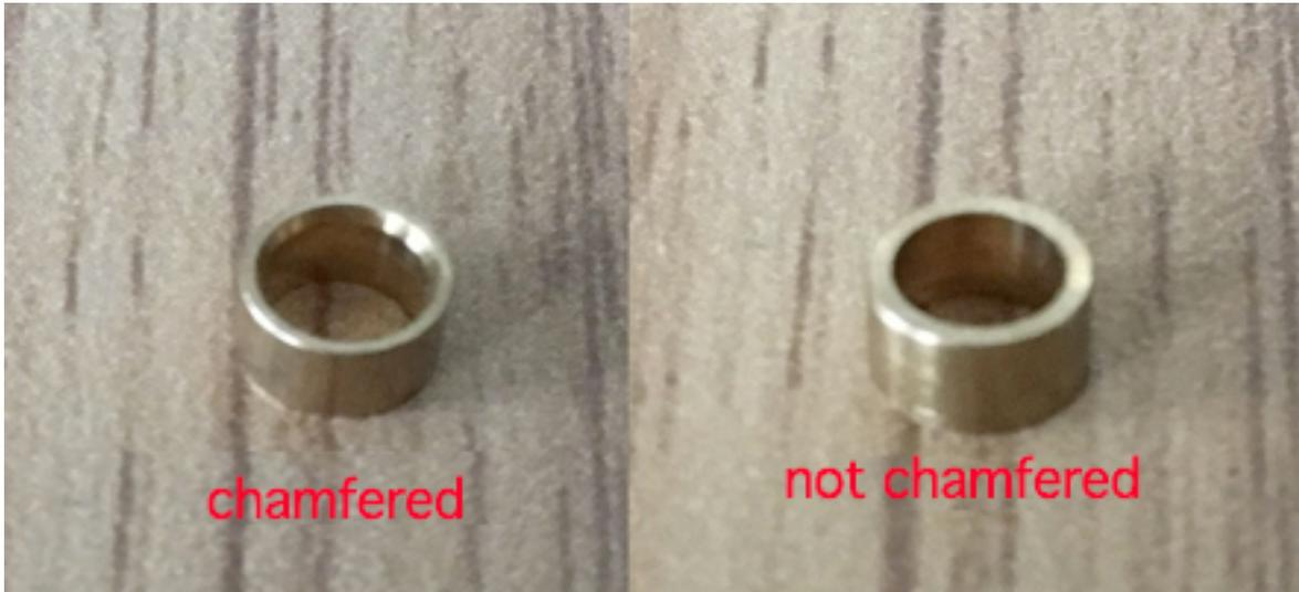
Get it through 1 (Bushings have a chamfering on one end. The chamfering end must be installed towards the nozzle direction to avoid tube from bursting. Follow the same method for next following assemblies).
