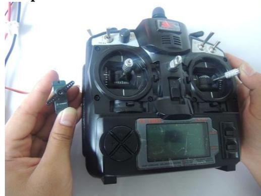
No additional adjustment required if it stays in horizontal position. Otherwise, you will need to adjust the button under the rocker towards left or right till the servo arms remains in the horizontal position.
