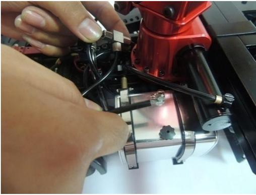
Take out the unconnected tube from the three tubes
