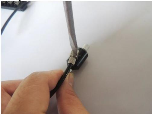
Use flat-blade screwdriver to fix 72 tightly.
