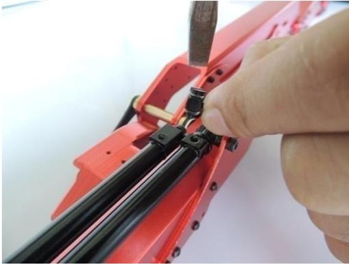
Use flat-blade screwdriver to install 2 onto cylinder
