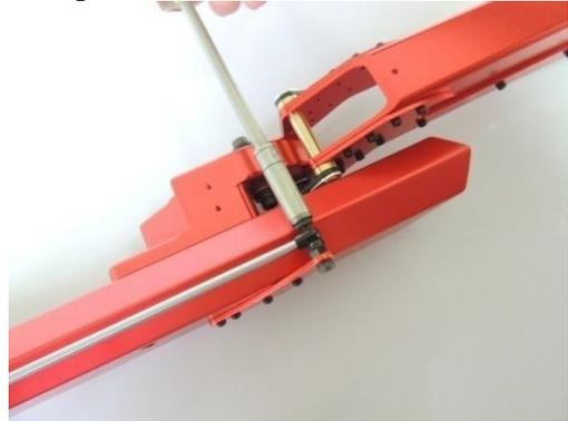
Use 5.5mm nut driver or pliers to lock tightly
