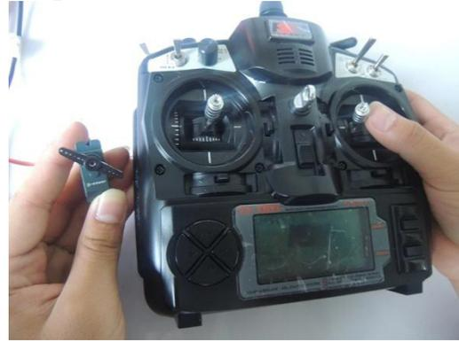
Adjust the servo to the left and right, up and down to make sure servo works normally. All servos should be checked like this.
