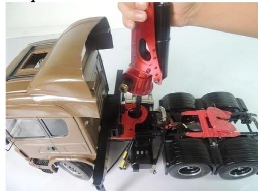
Put oil tube into the hole
