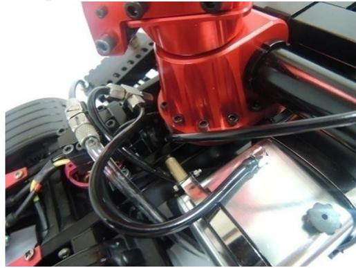
Install the tube on the oil tank like shown
