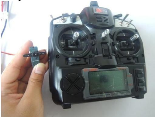
Try to keep the servo arm in the horizontal position as shown
