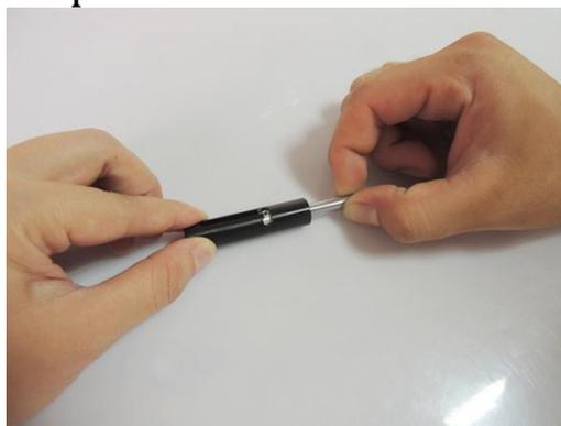
Push the inner small shaft out
