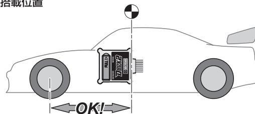
Mount as close to center of gravity (CG) as possible so that the yaw axis can be easily detected. Gyro sensitivity is reduced if placed behind the center of gravity (CG).
