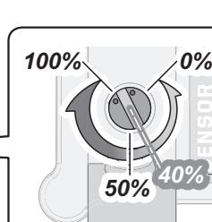
**Gyro sensitivity knob (Adjust gyro sensitivity)**
