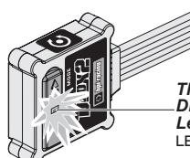
The LED will blink during initialization and will stop blinking when initialization is complete.
