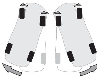
The drift assist system is correctly installed if the front tires are correctly adjusted in the direction the car is turning. If car is turning to the left, the front tires will rotate to the left. When turning right, the front tires will be turning to the right as well.
