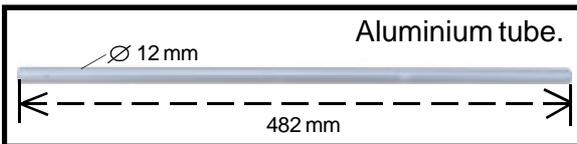
\*\*\* Test fit the aluminium tube dihedral brace into each wing haft. The brace should slide in easily. If not, use 220 grit sand around the edges and ends of the brace until it fits properly.
