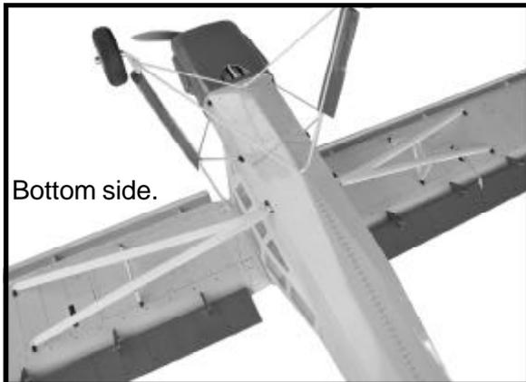
Plastic parts for bottom fuselage.
