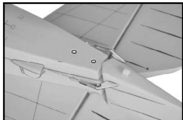
□ 3. Secure the tail wheel bracket in place using three 3mm x 12mm wood screws. Be careful not to overtighten the screws.
