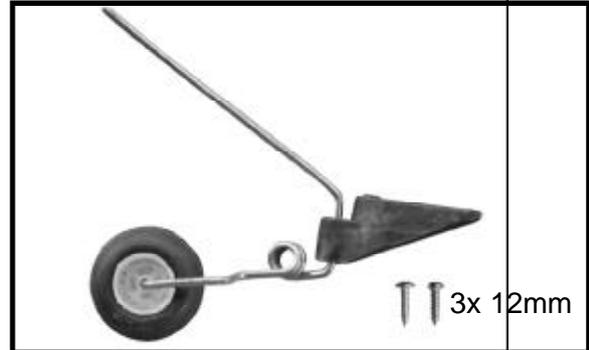
□ 2. Using a pen, mark the locations of the two mounting screws. Remove the tail wheel bracket and drill 1mm pilot holes at the locations marked.
