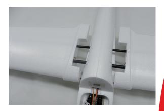
Now slide the carbon wing rods through the holes in the fuselage. Attach the wing to the fuselage. Make sure the servo cables are not pinched.
