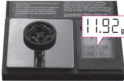
1 Put the diff (without oil) on the scale and check the weight (approximately 11.92g)
