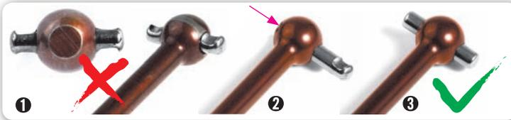
Do not use drive shafts when the pins are worn.
