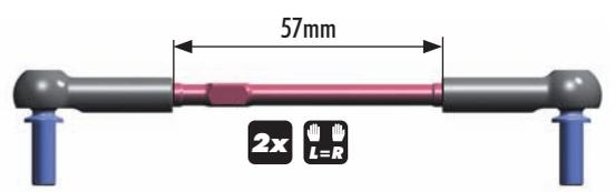
**TIP** Install the pivot balls with Professional Multi Tool (HUDY #183011)
