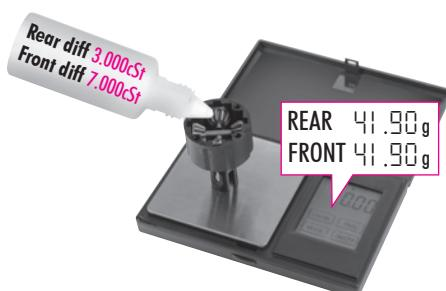
1. Put the diff (without oil) on the scale and check the weight:
