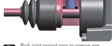
! Push joint against gear to remove gap.
