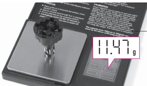
1 Put the diff (without oil) on the scale and check the weight (approximately 11.47g)
