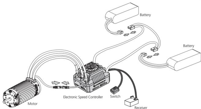
Refer to the wiring instructions and wiring diagram:
