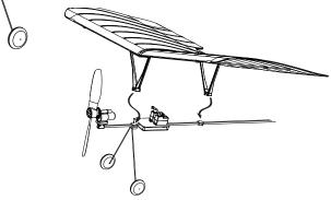
2. Install the main wing onto the fuselage by clipping the plastic mounts on the wing into the holders on the fuselage. Note the direction in the drawing. Make sure to fully push the mounts into the clips to prevent the wing from coming off during use. Make sure to re-check the fit of the mounts on the clips if you crash your plane.
