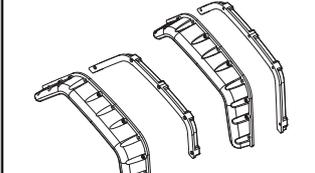
Front wheel panel (L+R) + Fixing strip of the front wheel panel (L+R)
