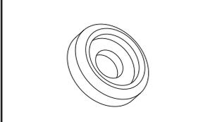
Fixing ring for the car shell bracket
