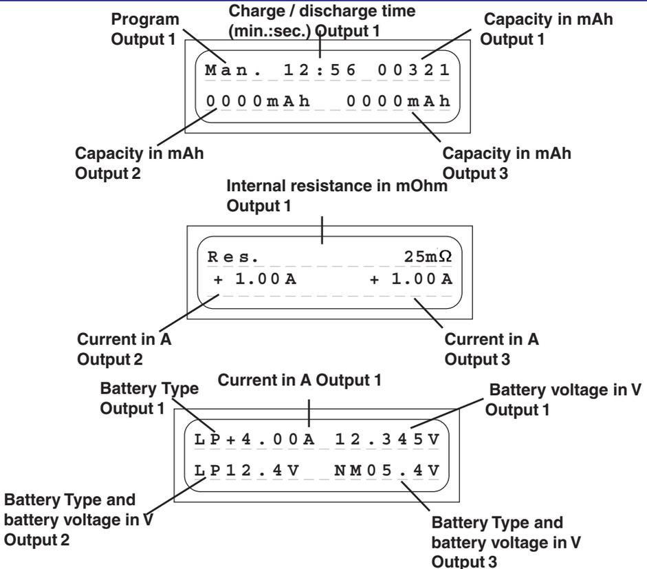
The two-line liquid-crystal screen displays in a clear form the important information generated during the charge / discharge process. The information remains visible on-screen until you disconnect the battery that is being charged. Once you connect another battery for charging, the previously displayed values are erased, and cannot be called up again.
