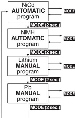
In the interests of clarity, the charge and set-up facilities of the ULTRA TRIO PLUS 14 are divided into four logical program groups.
