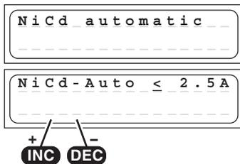
In this program the charger detects the type of Ni-Cd battery connected to it, and adjusts the charge current accordingly to avoid overcharging the pack. The maximum charge current can be set **before** you connect the battery to be charged. This is done using the INC / DEC buttons; the range available is 0.1 A to 5 A, or no restriction. The charge process is terminated automatically in accordance with the values already set for „Ni-Cd Delta Peak cut-off voltage“.
