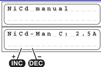
Select this program when you simply wish to recharge a battery using the set charge current. You can adjust the charge current using the INC / DEC buttons, but only **before** you connect the pack for charging. The range available is 0.1 A to 5 A. The charge process is terminated automatically in accordance with the values already set for „Ni-Cd Delta Peak cut-off voltage“.
