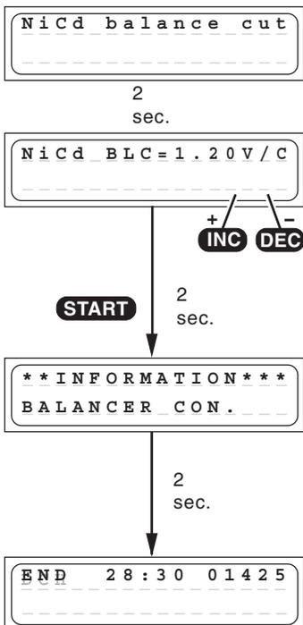
The discharge balancing program does discharge and balance up to 6 cells of a battery pack.
