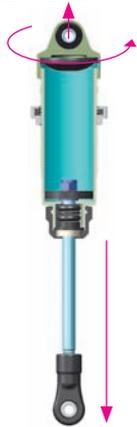
1 Extend the shock shaft completely and remove the shock cap.
