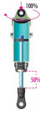
6 Keep the shock shaft pushed 50% into the shock body and tighten the shock cap completely. The rebound will be at approximately 50%.
