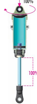
4 Gently place the shock cap assembly onto the filled shock body. Keep the shock shaft extended 100% from the shock body and tighten the shock cap completely. The rebound will be at approximately 100%.
