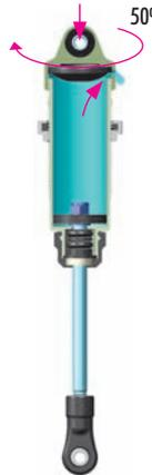
4 Gently place the shock cap assembly onto the filled shock body. Excess oil will spill from the shock.
