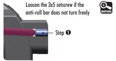
Loosen the 3x5 setscrew if the anti-roll bar does not turn freely
