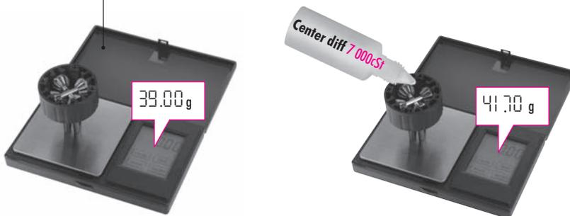
1. Put the diff (without oil) on the scale and check the weight (approximately 39g).
