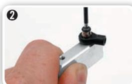
2 Tighten screw until pivot ball is tight against block.
