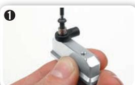
1 Place the pivot ball on the ball joint and use a screw to tighten it to an engine mount or some other part.
