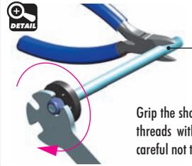
Grip the shock rod at top of exposed threads with side cutting pliers. Be careful not to damage the shock rod.
