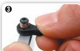
3 Lift ball joint until it snaps into place over pivot ball. Ball joint should move freely.
