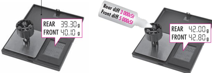
1. Put the diff (without oil) on the scale and check the weight:
