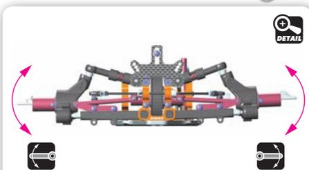
When the bars are set, verify that both sides move at the same time. If they do, the bars are set up correctly. If not, make sure that both downstops are the same and that the bar wire is flat.
