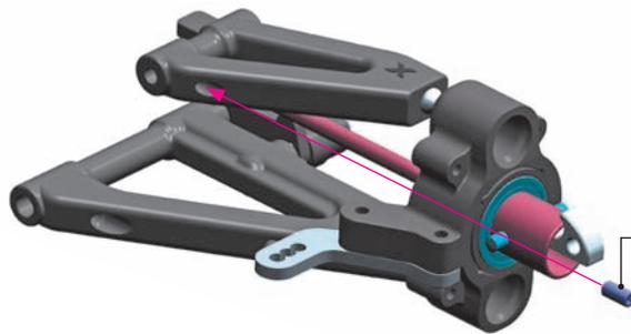
TIGHTEN GENTLY, tighten fully when the drive pins are assembled. (Page 29, step 1)
