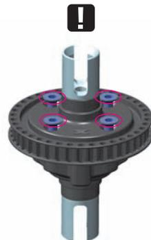
Tighten the screws equally but do NOT tighten them completely.
