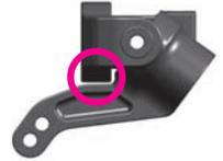
Attach servo arm to servo output shaft using screw from servo. Servo saver must be perpendicular to chassis when servo is in neutral.
