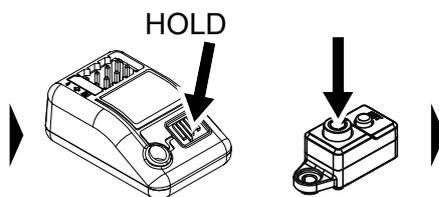
Press and hold the bind button on the receiver. Power on the receiver. The orange LED flashes, indicating the receiver is in bind mode. Release the bind button after the orange LED illuminates.
