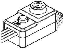
To reset all programming items, press and hold the set button for five seconds.
