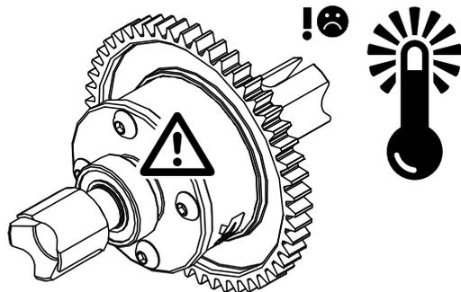
**! WARNING:** Do not hold handbrake button and activate forward or reverse at the same time. Center Differential may be damaged by doing this.
