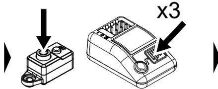
Power on the ESC. press the bind button three times quickly (within 1.5 seconds of the first button press).
