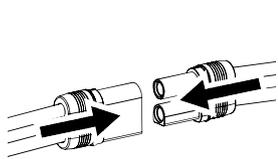
Connect a fully charged battery pack to the ESC.
