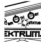
If battery status LED is flashing, the batteries need to be replaced.
