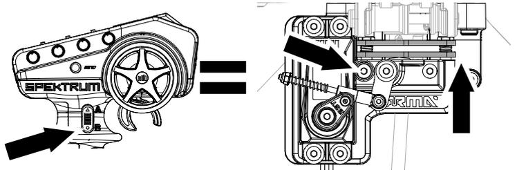
When the CH3 button is released all wheels spin freely.
