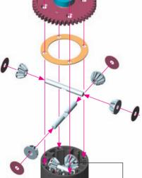
Fill to just above the satellite gears.
