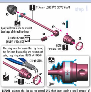
$\mbox{\bf BEFORE}$  inserting the clip on the central CVD shaft joint, apply a small amount of threadlock on the area where the clip goes.
