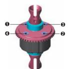
After assembly the differentials should have a length of 32.3 $\sim$ 32.5 mm measured from the ends of the installed ball-bearings. If differentials are longer, retighten the 4 screws holding the crown gears.
