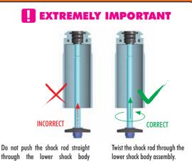
assembly; O-ring damage may result.
