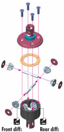
Silicone oil 7.000cSt Silicone oil 3.000cSt Fill just above the Fill just above the
