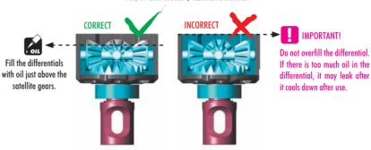
To ensure you have the same amount of oil from rebuild to rebuild, do the following:
