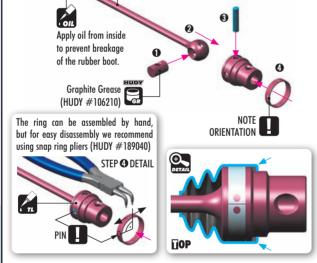
**BEFORE** inserting the clip on the central CVD shaft joint, apply a small amount of threadlock on the area where the clip goes.
