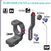
We recommend using the composite shim to create a bigger surface that touches the body; this will help prevent paint from being removed from the inside of the bodyshell. Before inserting the screw, use CA glue to seal & strengthen the outside edges of the upstop. Insert the screw carefully.
