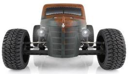
Factory-finished body with integrated LED lights, 2 front, 2 rear
