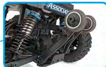
Four-position adjustable wheelie bar
