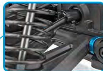
Heavy duty, hardened steel CVA axles
