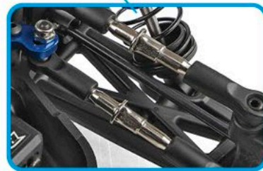
Turnbuckles to adjust camber and toe
