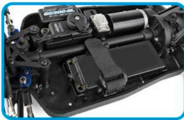
Molded tub chassis with covered center driveshaft
